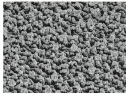
毛面处理铜箔：Peak Type for Matte-treated side
