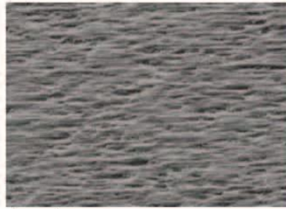
光面处理铜箔：Peak Type for Shining-treated side
